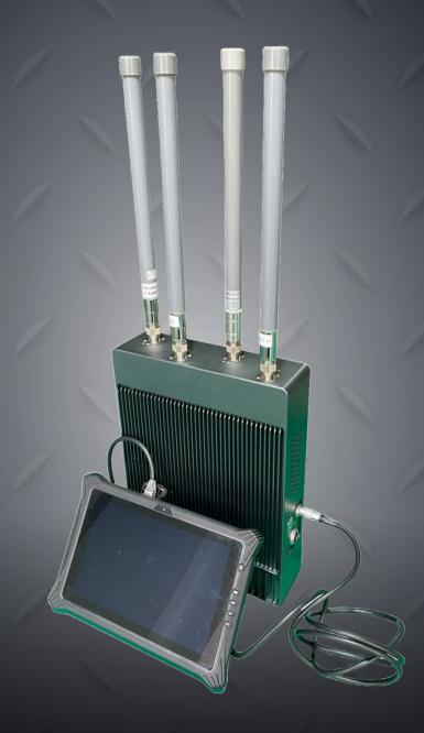
The I-Meta AI Versatile Portable Tracer is a portable drone detection and localization device. Utilizing AI, protocol analysis, and spectrum analysis, it identifies and tracks consumer drones efficiently. Designed for mobility and rapid response, it offers comprehensive drone detection capabilities.
