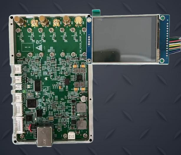
Designed for handheld or portable jamming devices, our drone detection module excels in identifying racing drones, DIY drones, and the full range of DJI drones within a 1-3 km radius. It triggers audio-visual alarms upon detection and ensures covert, easy operation through spectrum and protocol analysis.
